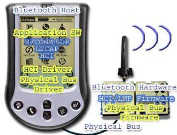
Fig. 1. Components of a Bluetooth™ System
